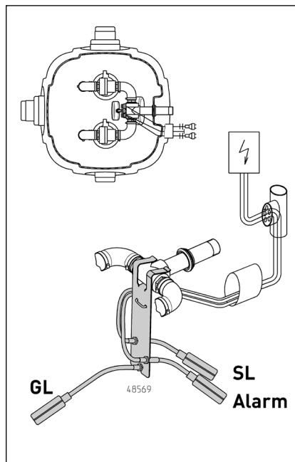
GL-Base load | Alarm | SL-Peak load
