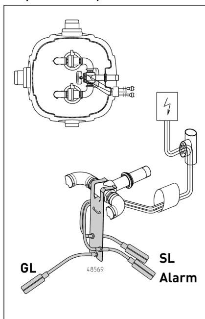
GL-Basisbelasting | Hoogwateralarm | SL-Piekbelasting
