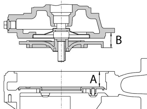
4. Measure dimension B on each blade and note the largest measurement.
